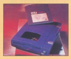
The Zip from lomega is a removable cartridge system that is fast increasing in popularity. It has an almost magical ability to fit just under 100Mb of data onto cartridges that are only marginally bigger than floppies. Could this be the end of the floppy as we know it?
