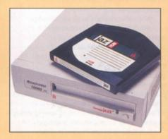
The Jaz drive is the big brother of the Zip and is also cartridge-based. However, its cartridges are a bit bigger – understandable when you consider that they can contain up to 1Gb of data! This drive is a superb asset for multimedia production.
